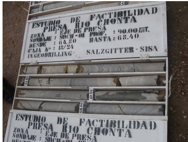
Photo 2. Rock sample from geotechnical studies in the area of the dam axis.
